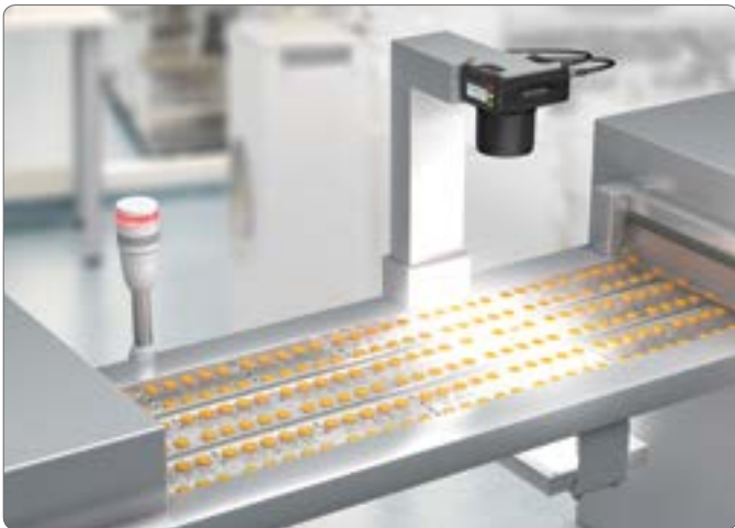
Blister pack inspection using BLOB Tool
