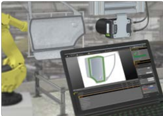
Door panel adhesive inspection using Bead Tool
