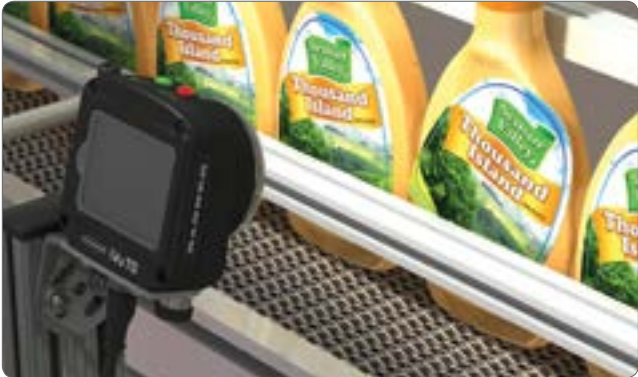
Label detection using a Match Sensor
