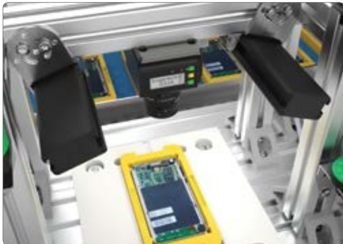
Cell phone inspection using Measure and Match Tools
