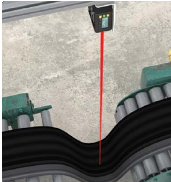
Loop control on a calendering machine
