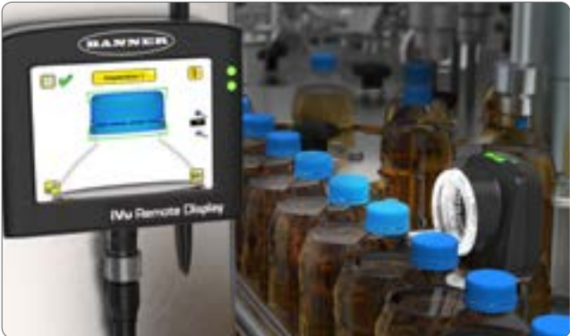
Cap verification using a Color Area Sensor
