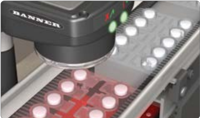
Blister pack inspection using an Area Sensor
