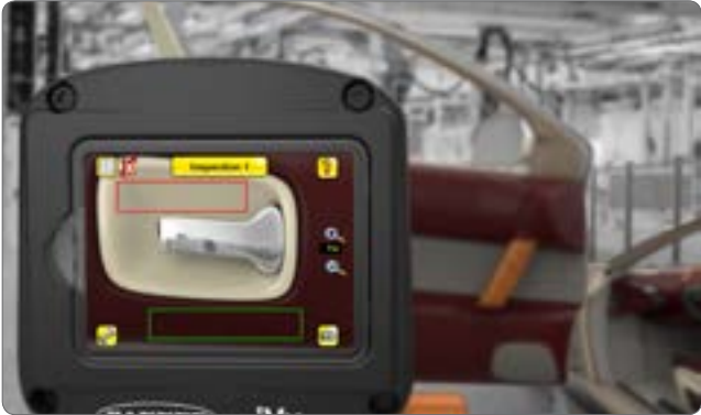
Trim color verification using an Average Color Sensor
