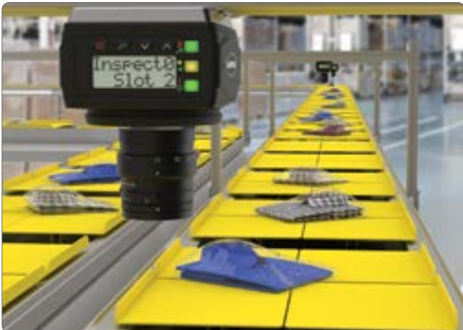
Empty sortation conveyor inspection using Blemish Tool
